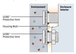
The Gore proprietary membrane is constructed of ePTFE and allows for the free passage of gases and vapors while at the same time preventing liquid and particulates from entering the housing.
